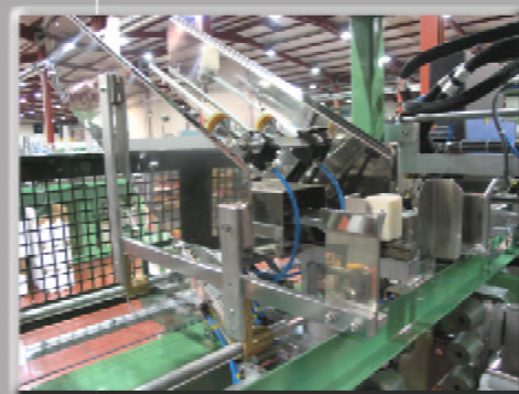
END PANELS FEEDER
