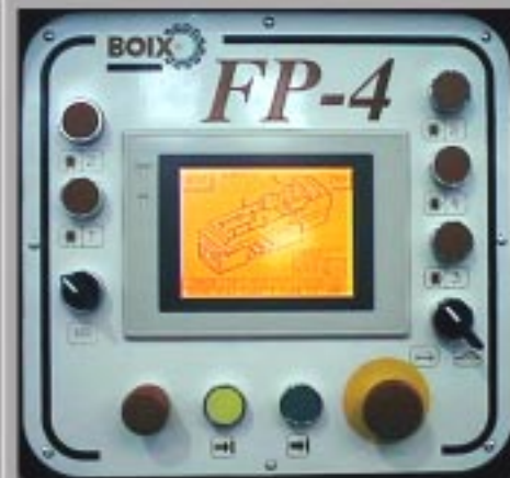
CONTROL PANEL WITH PROGRAMMER NT30
