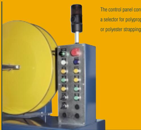
The control panel contains a selector for polypropylene or polyester strapping.
