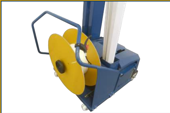
New ergonomic handle equipped with brake release lever
